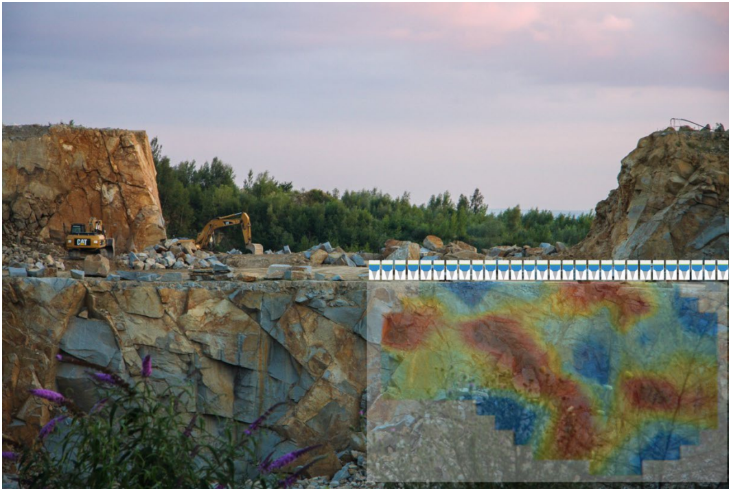
Figure 1: Schematic image of a working quarry with example SmartSolo node deployment that provide continuous vibration monitoring and (time-lapse) velocity imaging (superimposed colour tomography velocity variation image). Photo by Kurt Bouda from Pixabay .
