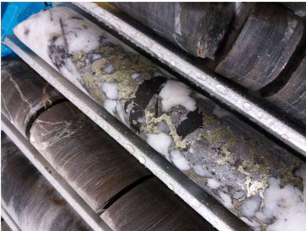
Figure 1: Strong copper and tungsten mineralisation in diamond drill core from Redmoor.
