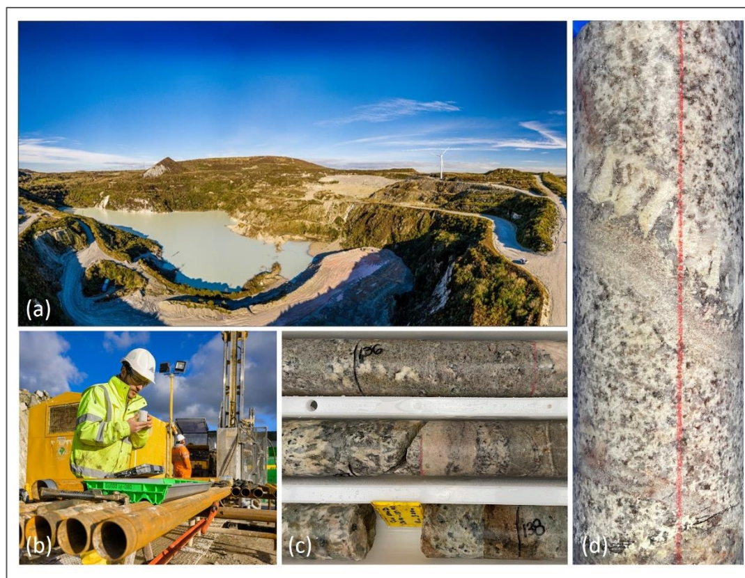
Figure 1: (a) Overview of Imerys British Lithium Gunheath Project site, looking NW; (b) geologist inspecting diamond drill core; (c) drill core showing mineralogical and textural variation in granite contact zone; (d) drill core specimen of typical 'G5' topaz granite containing thin pegmatite-aplites.
