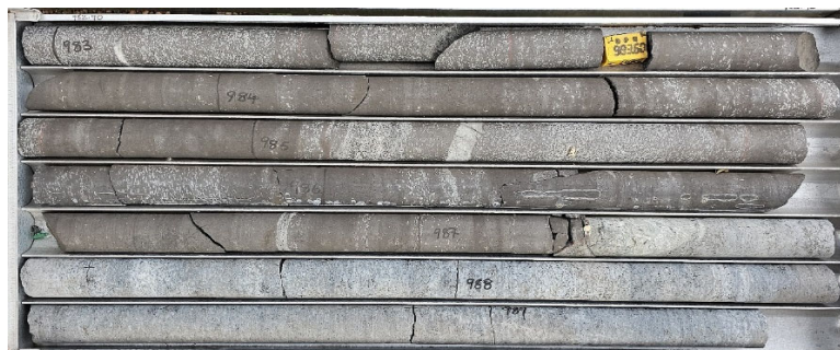
Figure 1: Main magnetite layer in one of the Mokopane drill cores to be studied, using petrographic and geochemical methods.
