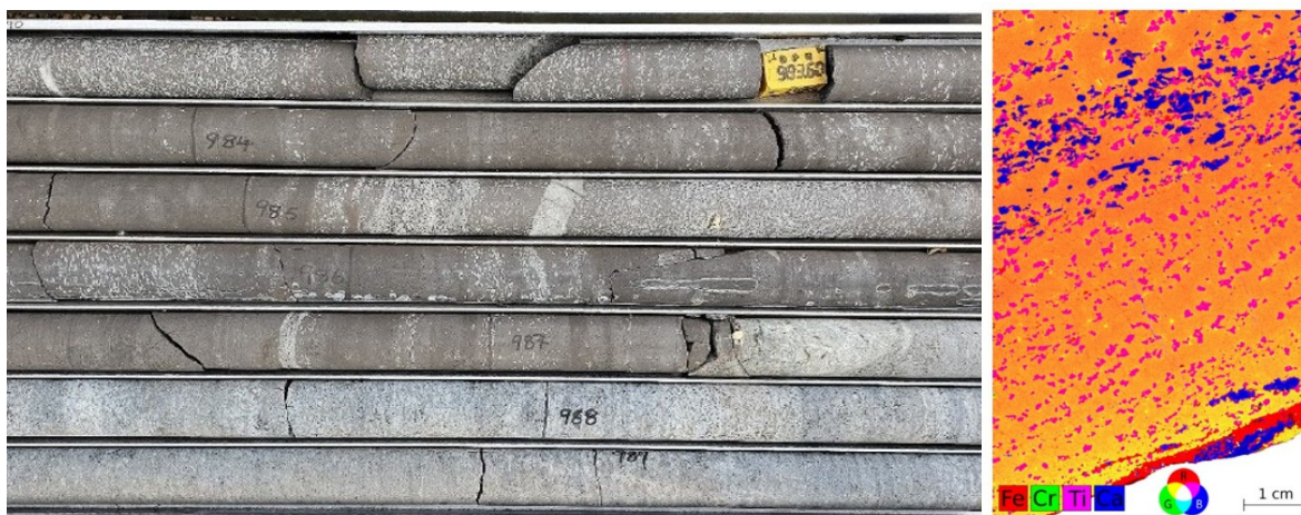
Figure 1: (left) Main magnetite layer in drill core to be studied, (right) MicroXRF image of magnetite layer (Nikonow et al. 2026).
